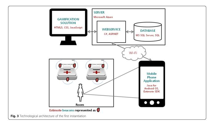
these signals, the application was able to detect if it is near the beacon or not. For example, if the application detects strong signals from a beacon placed in a sink, then it will know that the HCW is near that sink. This information was continuously processed using the already mentioned algorithm (which implements the model from Fig. 2), and every time an HH moment was detected and validated (or not), the application sent this information to a web service, which in turn updated the database.
